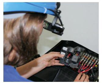
Augmented reality providing worker instructions; Source: Fraunhofer IFF
