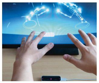
Hand movement tracking with sensors such as the Leap Motion<sup>®</sup> 3D Controller; **Source:** Fraunhofer IFF
