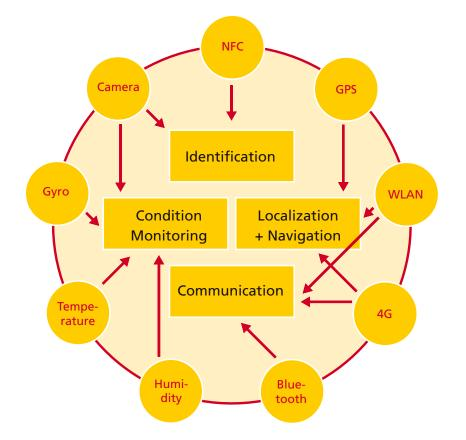
Figure 5: Sensor technologies in current mobile devices and how they can be applied in logistics; Source: Fraunhofer IFF
