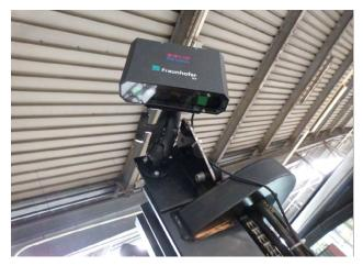
A range imaging sensor in an ebedded system with an industrial housing; **Source:** Fraunhofer IFF
