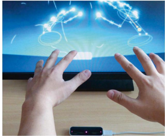
Hand movement tracking with sensors such as the Leap Motion® 3D Controller; **Source:** Fraunhofer IFF
