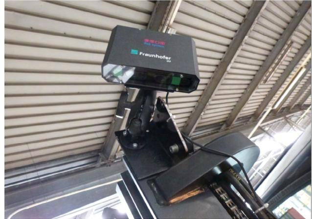
A range imaging sensor in an embedded system with an industrial housing; **Source:** Fraunhofer IFF
